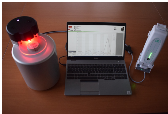
Figure 1: A picture of the PDM with a glass plate present, connected to the software.
