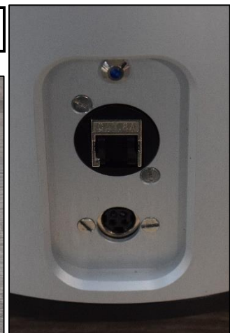
I/O Interconnection socket with power inlet
