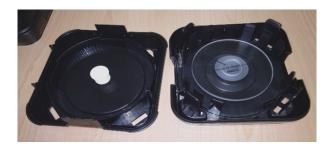
Important for sampling and transportation of the samples are the exposure boxes. These boxes cover the witness plate and preserve the state of exposure after the gathering of the sample. Boxes can be as well used to transport blank premeasured disks to a test location. As the witness plate is detachable and many boxes can be exposed at the same time, parallel measurements are possible. The sampling box allows as well measurement schemes per part of a day night.
