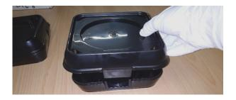
Exposure boxes can also be used by volunteers exposing the boxes i.e. for a few hours. This makes it possible to carry out a simultaneous field test over a large area with lots of measuring points. Handling and data processing are made easy.
