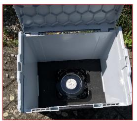
around he bottom part of the exposure box was used as Stokes Chamber.
